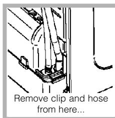
Remove the existing clip and hose from position shown (*see diagram*).
