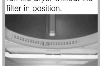
**!** Failure to clean the filter after EVERY drying cycle will affect the drying performance of your machine.
