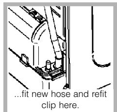
Fit a suitable length of hose to the new location shown (*see diagram*) and refit clip.
