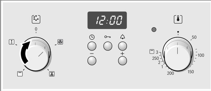
2. Use the temperature selector to set the temperature or the grill setting.
