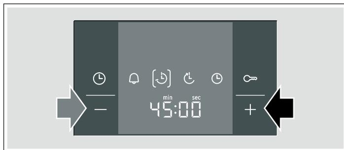
The main oven will start up after a few seconds. The cooking time counts down in the display and the
