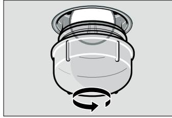
3. Replace the oven light bulb with a bulb of the same type.
